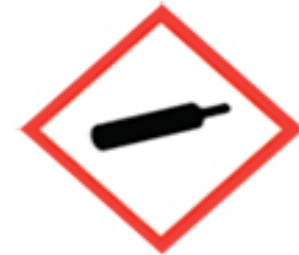
Gas under pressure
