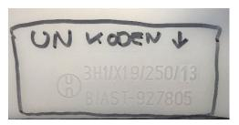
Example from a 5-liter plastic jerrican: It is UN approved, it is X-quality, and it was manufactured in 2013, which means that in 2023 it **cannot** be used for chemical waste!
