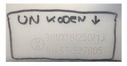
Example from a 5 liter plastic jerrican: It is UN approved, it is X-quality and it was manufactured in 2013, which means that in 2021 it **cannot** be used for chemical waste!
